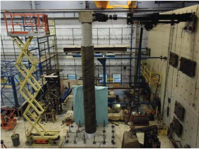
**Fig. 4.** Global view of Specimen S5 [76.2-cm (30-in.) diameter] ready for test.
